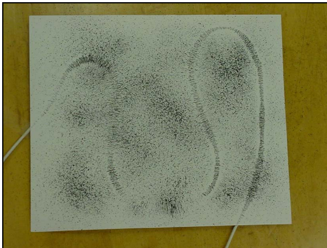
Figure 1: Iron filings align with the magnetic field generated from electric current flowing in the wire hidden beneath the paper.
